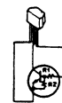
DTC114ES (R1=10K, R2=10K) DTC114YS (R1=10K, R2=47K) DTC124ES (R1=22K, R2=22K) DTC144WS (R1=47K, R2=22K)
